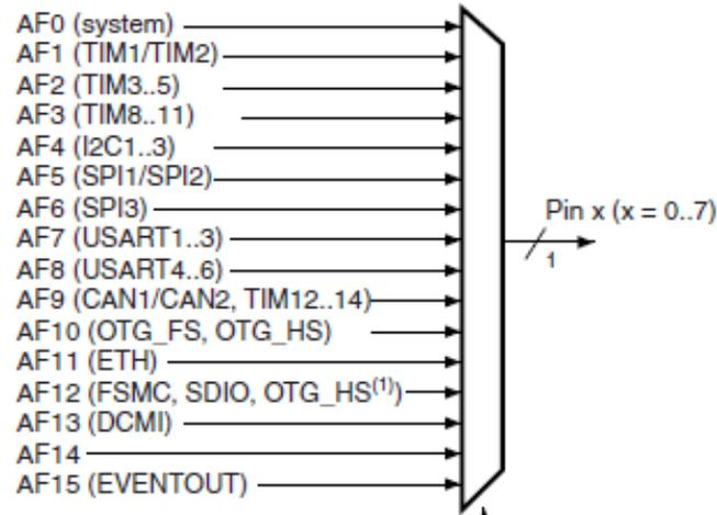
For pins 8 to 15, the GPIOx\_AFRH[31:0] register selects the dedicated alternate function
