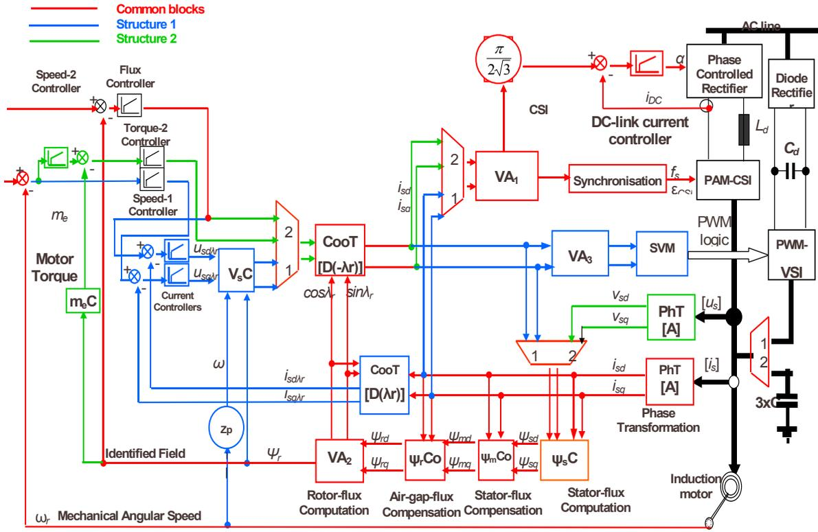
Fig.2. Reconfigurable Rotor-Field Oriented Vector Control System with Space Vector Modulation (SVM) for the tandem converter-fed induction motor.
