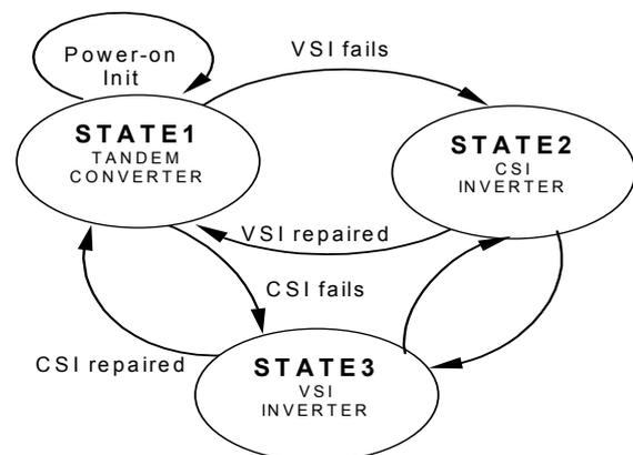
Fig. 1. The state transition graph of the tandem converter system.
