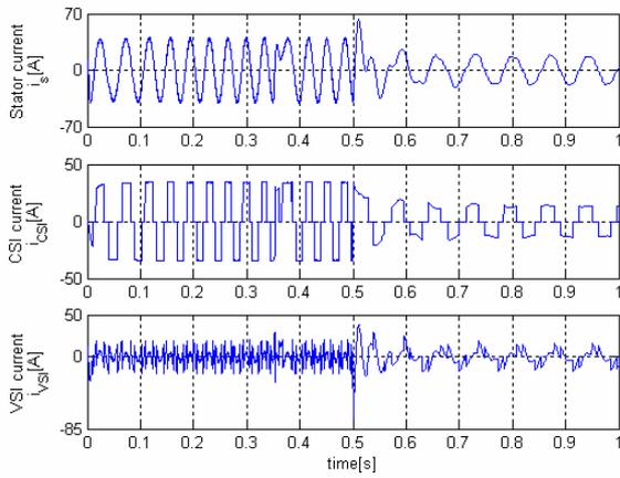
Fig. 5. Current waveforms before and after reconfiguration.
