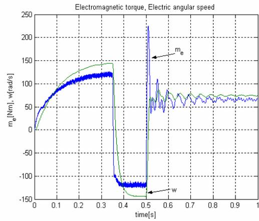
Fig. 6. Electromagnetic torque, electric angular speed before and after reconfiguration.
