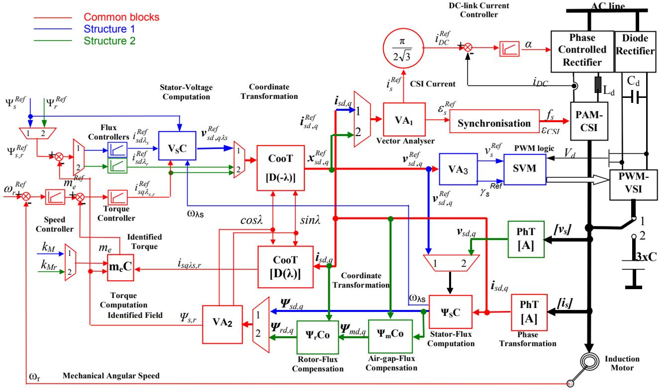
Fig. 3. Vector control system with reconfiguration of stator-field orientation and space vector modulation (SVM) for the tandem converter-fed induction motor.
