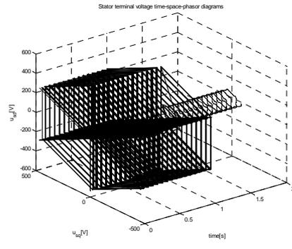
Fig. 14. Stator terminal voltage space-phasor diagrams.
