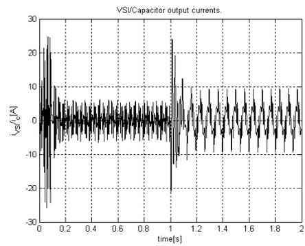
Fig. 8. VSI/Capacitor output currents.
