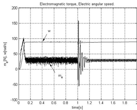
Fig. 5. Electromagnetic torque, Electric angular speed.
