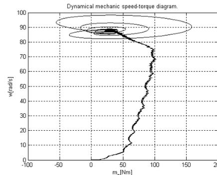
Fig. 6. Mechanical characteristics of the induction machine
