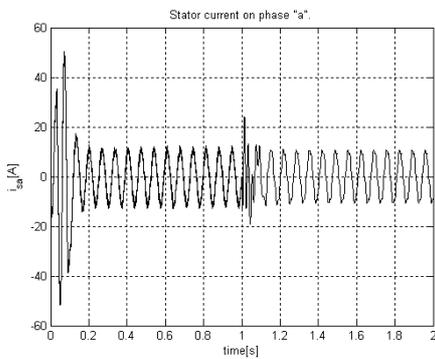
Fig. 7. Stator current on phase "a".
