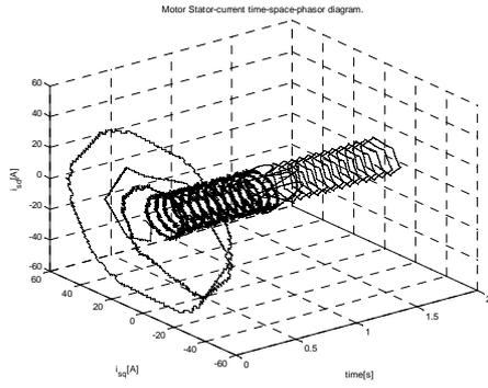
Fig. 9. Motor Stator-current space-phasor diagrams.
