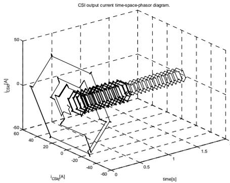
Fig. 10. CSI output current space-phasor diagrams.
