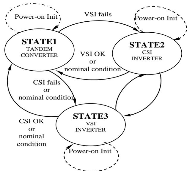
Fig. 1. The state transition graph of the tandem converter system
