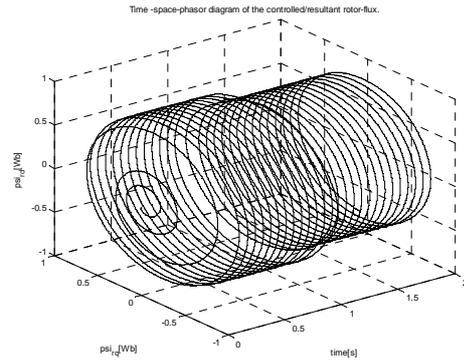
Fig. 12. Space-phasor diagrams of the controlled/resultant rotor-flux.
