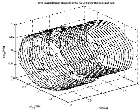
Fig. 13. Space-phasor diagrams of the resulting/controlled stator-flux.
