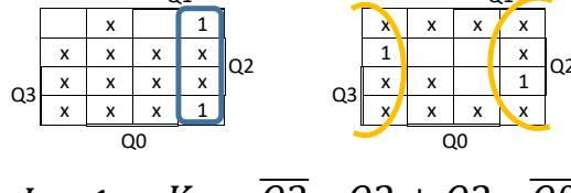
$$J_1 = 1 \quad K_1 = \overline{Q3} * Q2 + Q2 * \overline{Q0} + \overline{Q3} * \overline{Q0}$$
