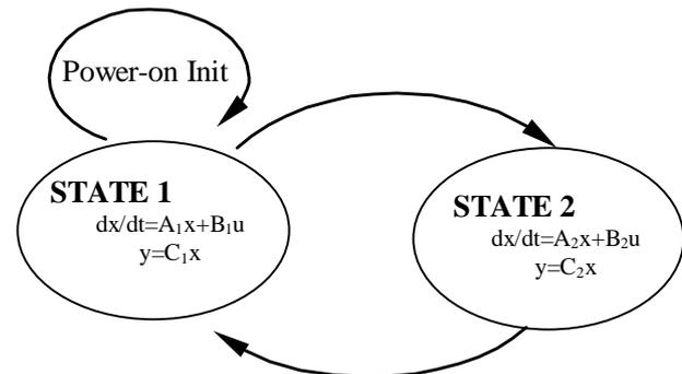
Fig. 3. The state transition graph of the re-configurable controller
