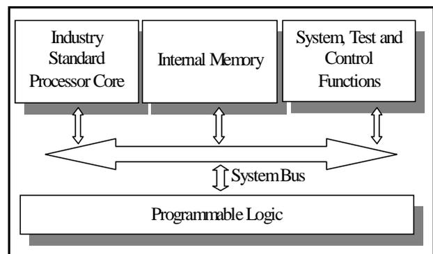
Fig. 2. Structure of the Triscend CSoC
