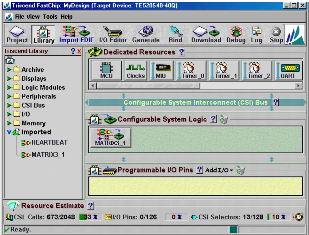
Fig. 5. 33% of Resources used in the CSL implementing the matrix multiplication
