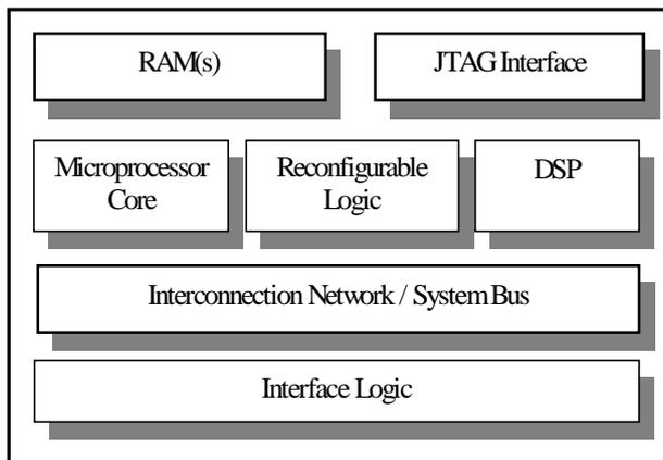
Fig. 1. Possible structure of a future Field Configurable System on a Chip
