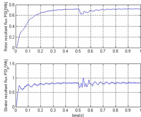
Fig. 6. Rotor and stator resultant flux.
