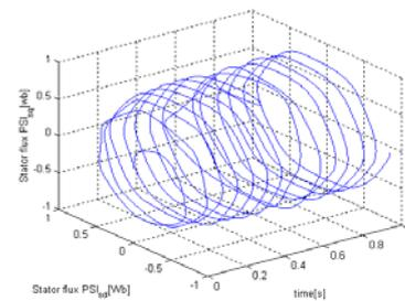
Fig. 11. Stator-flux space phasor.
