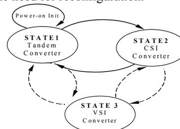
Fig 1. Reconfigurable state machine with different vector control structures in each state
