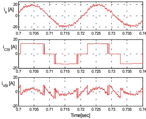
Fig. 3. Current waveforms at the output of the tandem converter.
