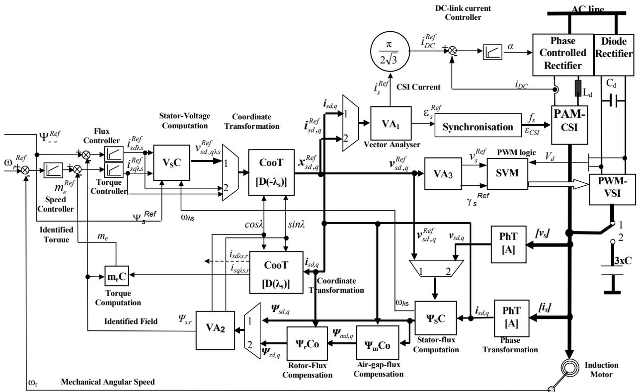
Fig. 2. Stator-field-oriented vector control system for the tandem converter-fed induction motor
