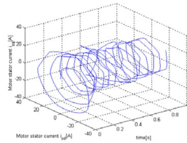
Fig. 10. Motor current stator space phasor
