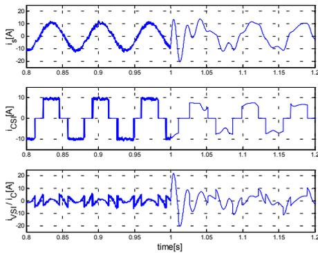
Fig. 9. Simulated current waveforms before and after reconfiguration.
