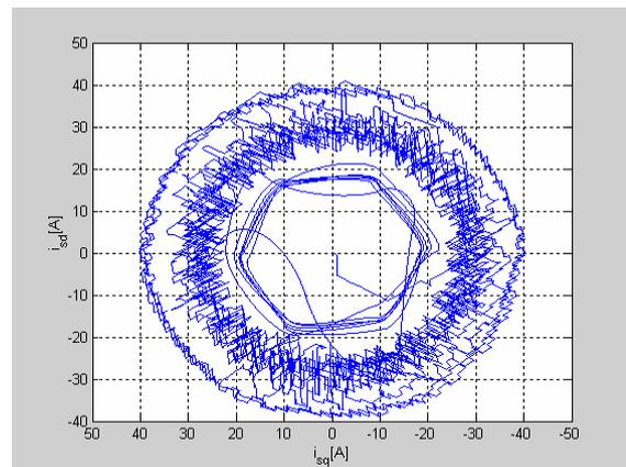
Fig. 5. Stator-current space-phasor.
