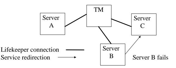
LifeKeeper service runs on each server and maintains a heartbeat connection so it can detect and respond to server failures. The TM replicates application logic within and across servers for scalability and ensures continued access to services from either server in case of component failures.
