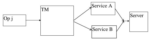
TP monitors' *funnelling* capabilities allow large number of clients to share scarce system resources on nodes. This idea of sharing is based on the statistical fact that not all clients want to perform transactions exactly at the same time.
