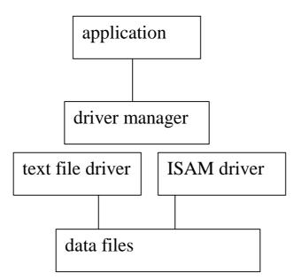
The driver should perform the DBMS functions, it replaces the missing DBMS
