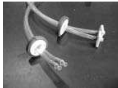
Figure 1: Acoustic wave guides and their suspension arrangement
