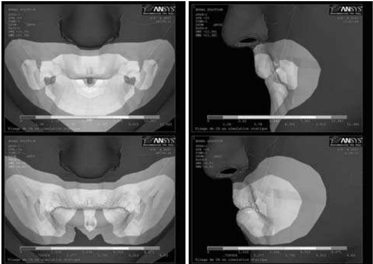
Figure 3 Simulation of the Orbicularis Oris contraction, without (top panels) and with (bottom panels) handling of lips-teeth and upper-lip/lower-lip contacts.
