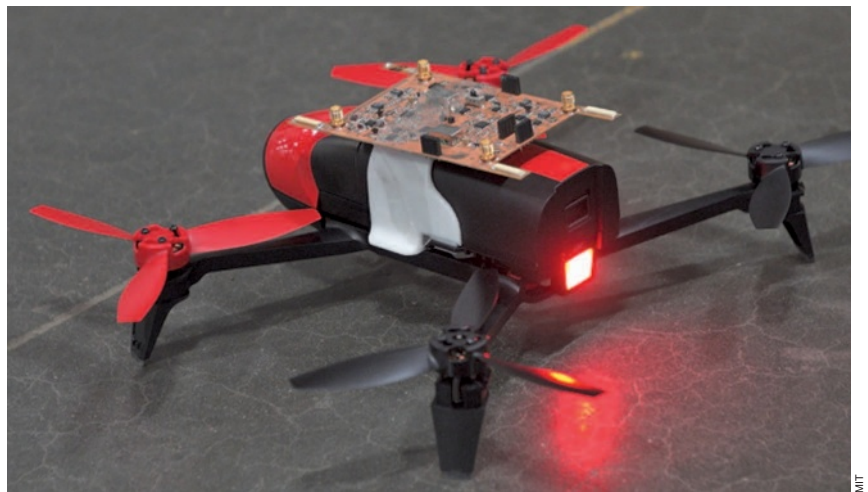
FIGURE 1. The RFLy drone and relay circuit.
