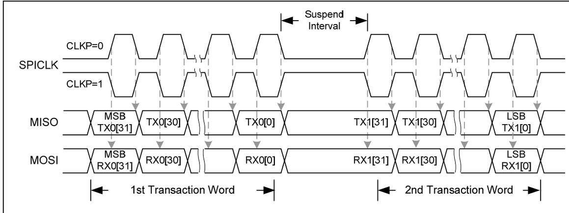
Figure 5-55 Two Transactions in One Transfer (Burst Mode)
