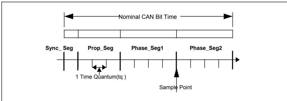
Figure 5-82 Bit Timing
