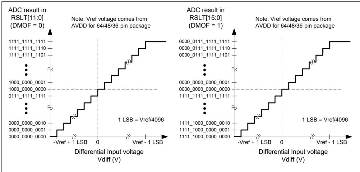
Figure 5-107 ADC differential input conversion voltage and conversion result mapping diagram
