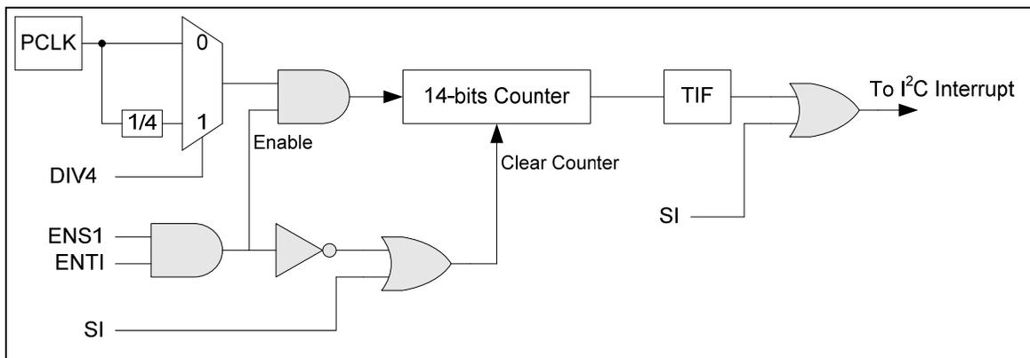
Figure 5-26: I<sup>2</sup>C Time-out Count Block Diagram
