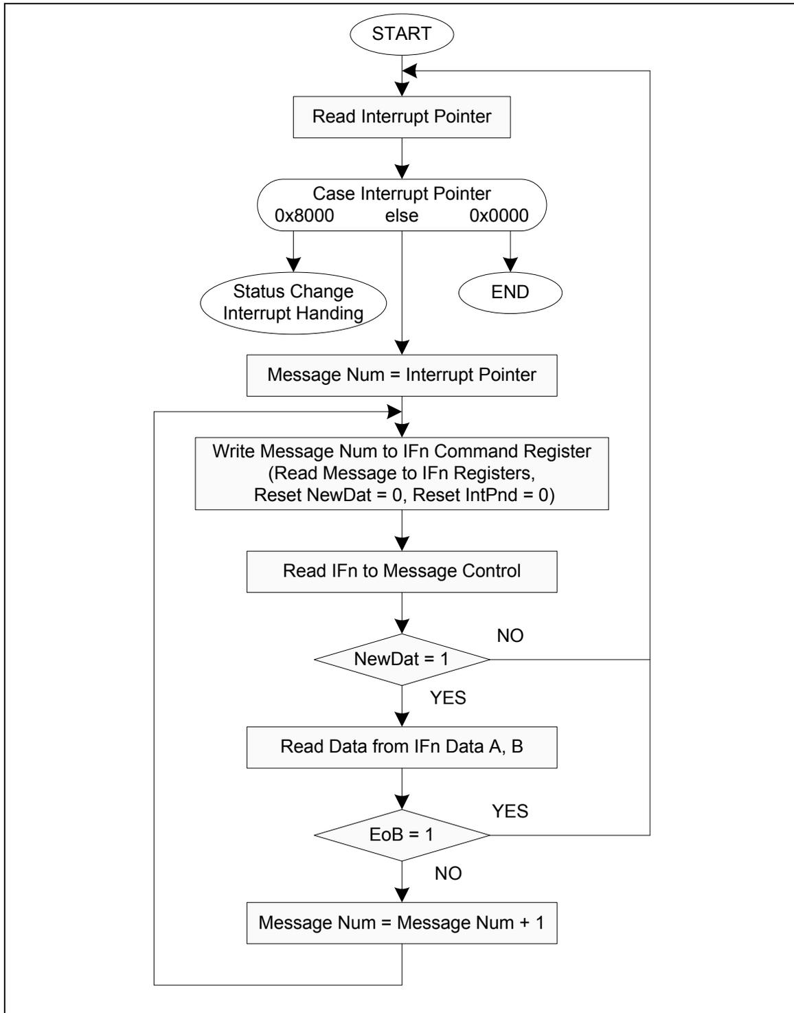
Figure 5-81 Application Software Handling of a FIFO Buffer
