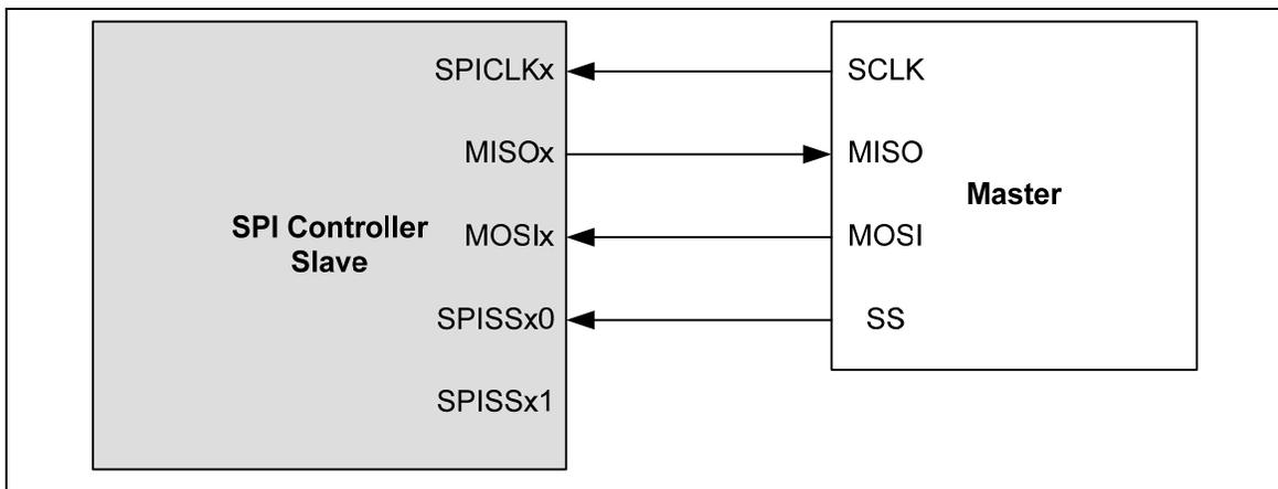
Figure 5-52 SPI Slave Mode Application Block Diagram
