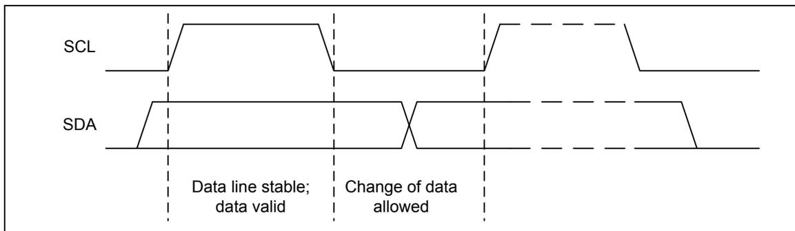
Figure 5-23 Bit Transfer on the I<sup>2</sup>C bus
