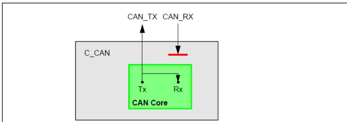
Figure 5-78 CAN Core in Loop Back Mode
