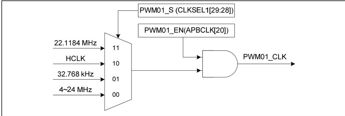
Figure 5-33 PWM Generator 0 Clock Source Control
