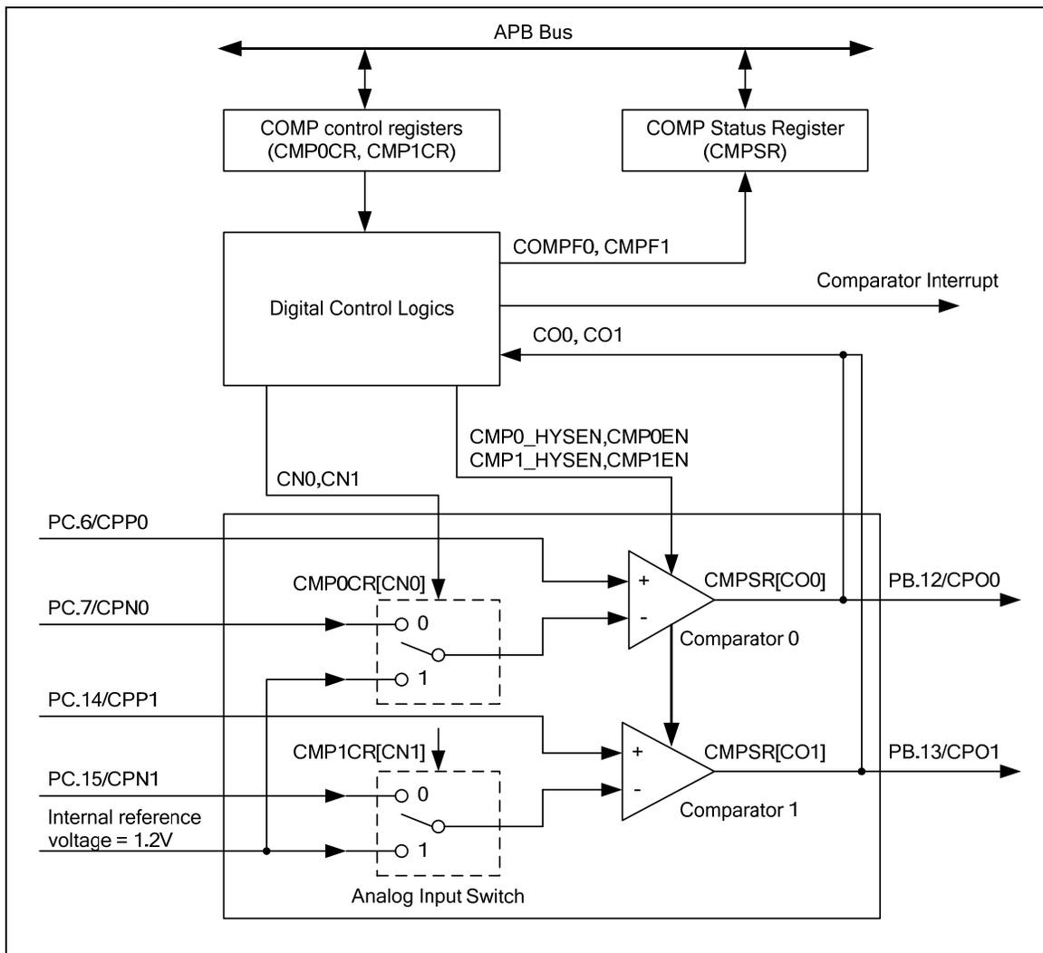
Figure 5-108 Analog Comparator Block Diagram
