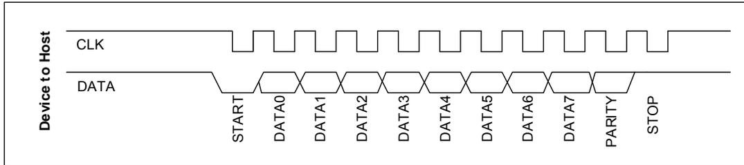
Figure 5-88 Data Format of Device-to-Host
