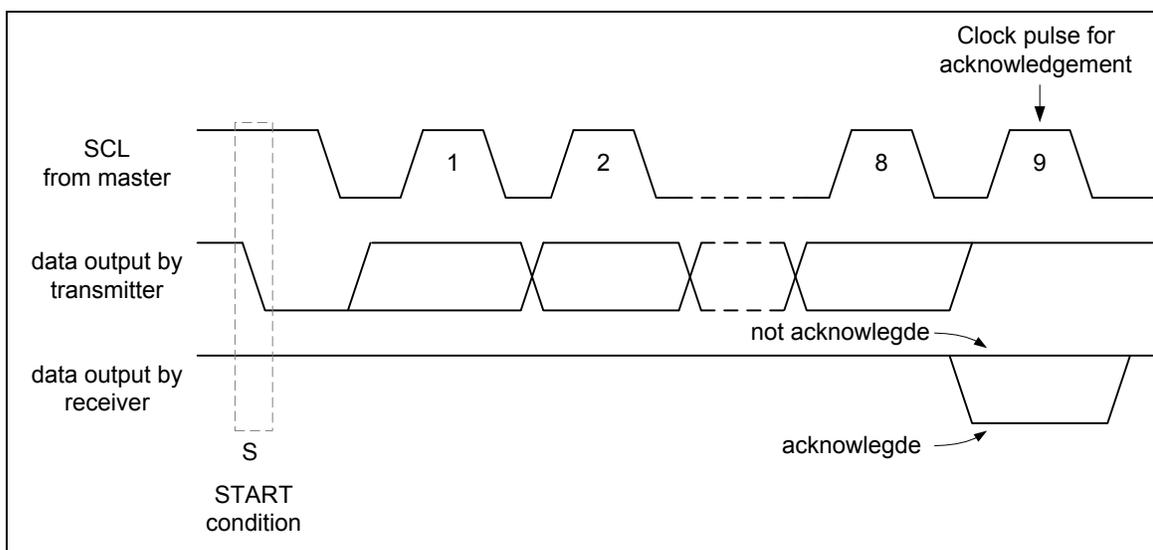
Figure 5-24 Acknowledge on the I<sup>2</sup>C bus
