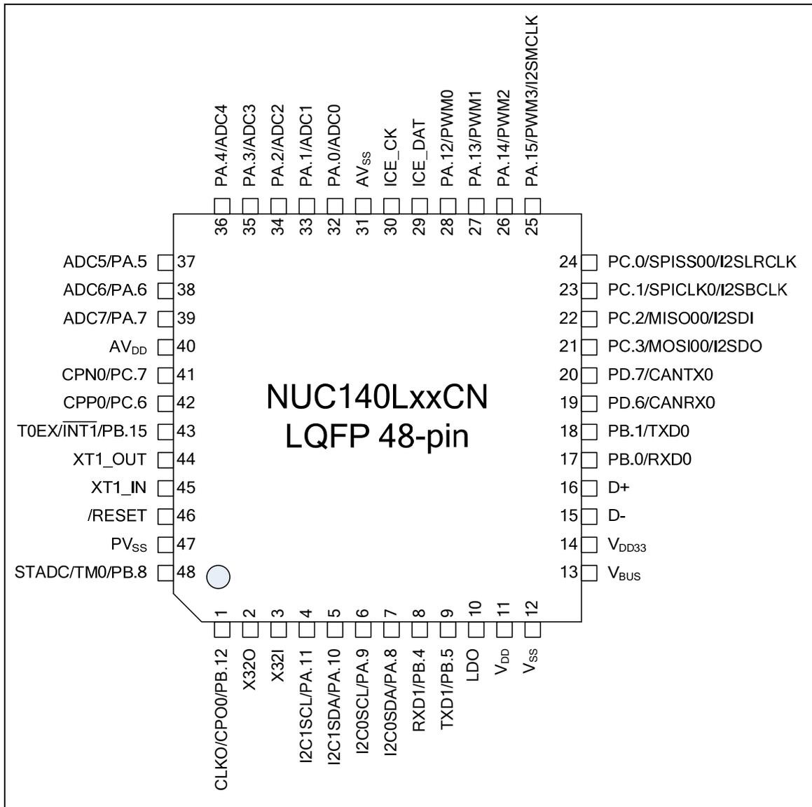
Figure 3-7 NuMicro™ NUC140 LQFP 48-pin Pin Diagram
