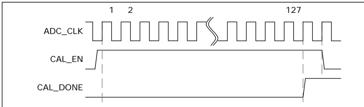
Figure 5-99 ADC Converter Self-Calibration Timing Diagram
