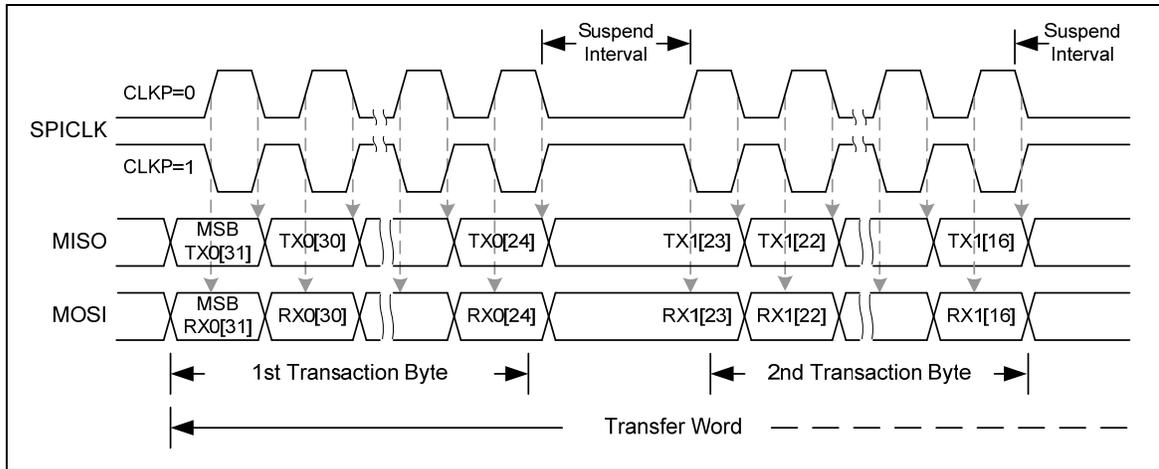
Figure 5-57 Timing Waveform for Byte Suspend
