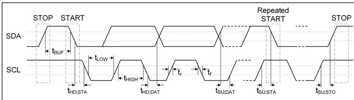
Figure 5-18 I<sup>2</sup>C Bus Timing
