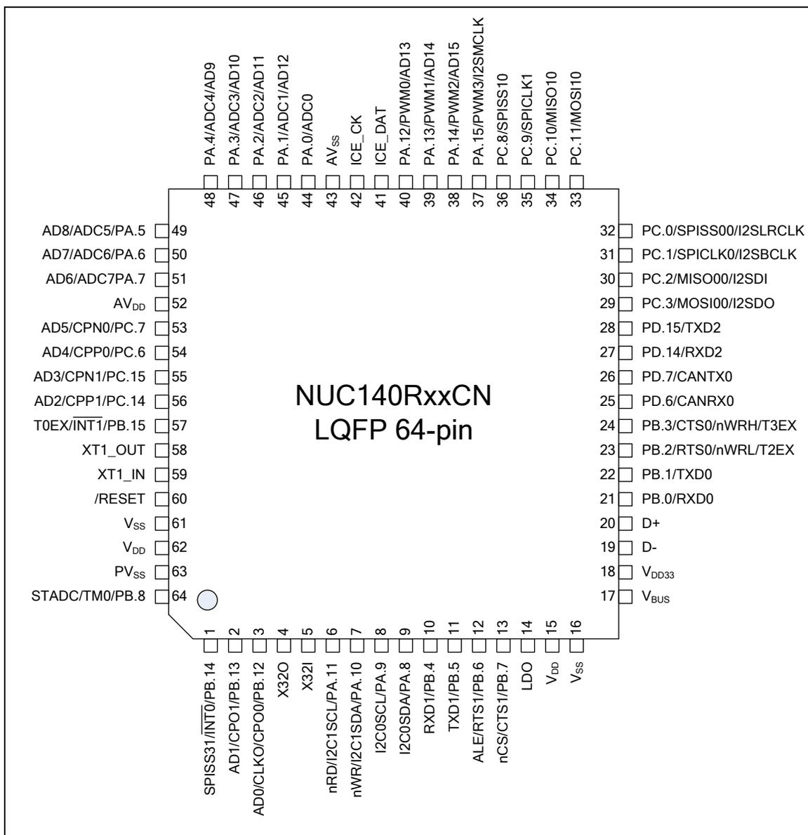
Figure 3-6 NuMicro™ NUC140 LQFP 64-pin Pin Diagram
