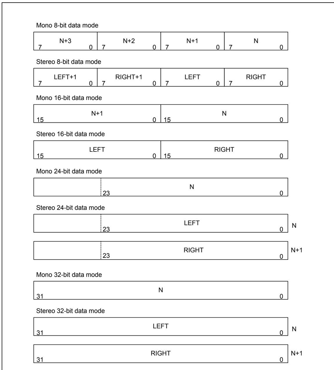
Figure 5-97 FIFO contents for various I<sup>2</sup>S modes
