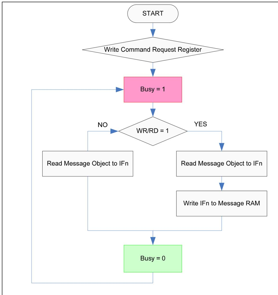
Figure 5-80 Data transfer between IFn Registers and Message
