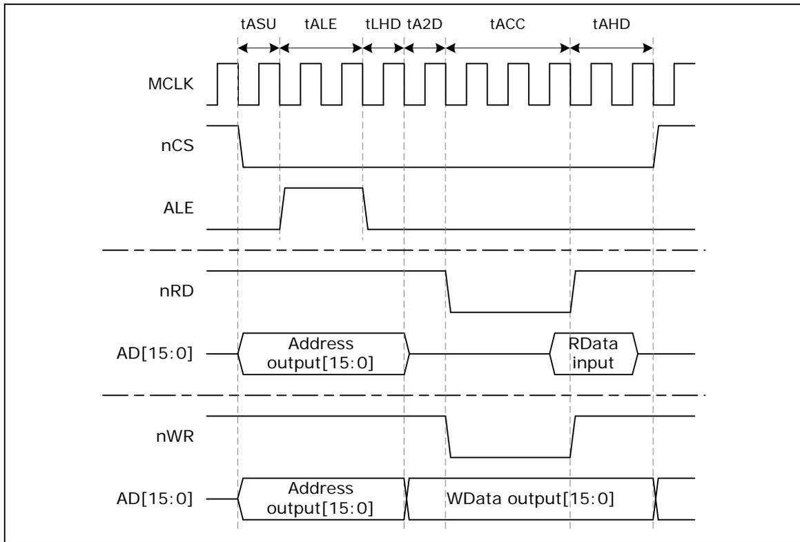
Figure 5-114 Timing Control Waveform for 16-bit Data Width
