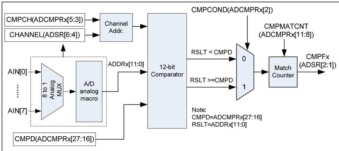
Figure 5-104 A/D Conversion Result Monitor Logics Diagram
