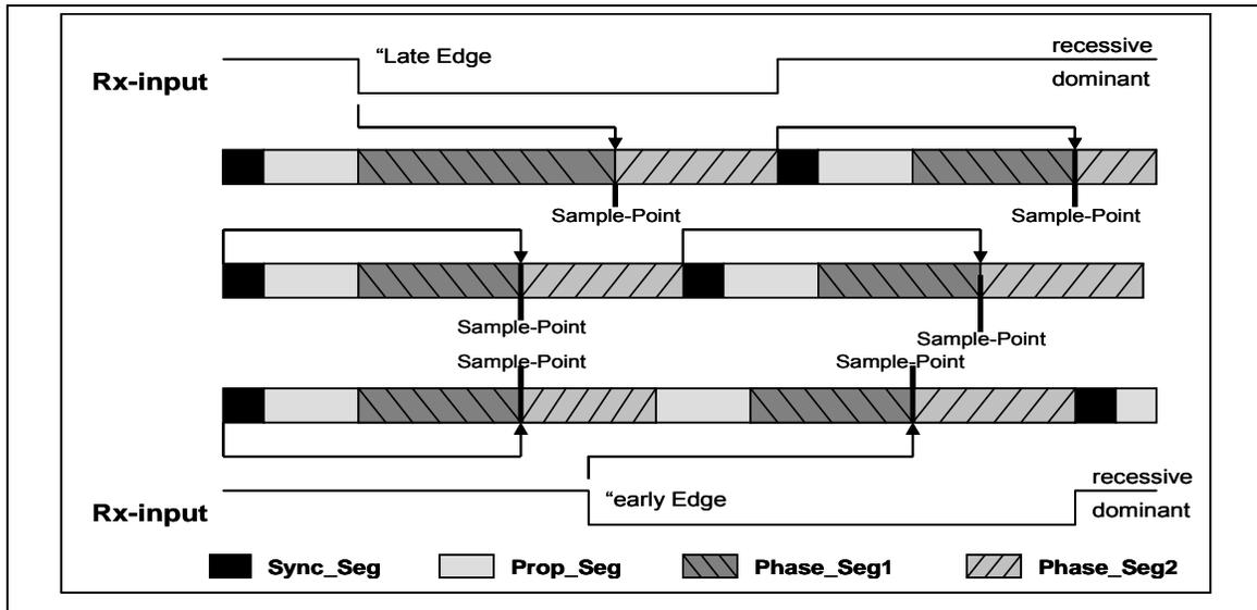
Figure 5-84 Synchronization on “late” and “early” Edges
