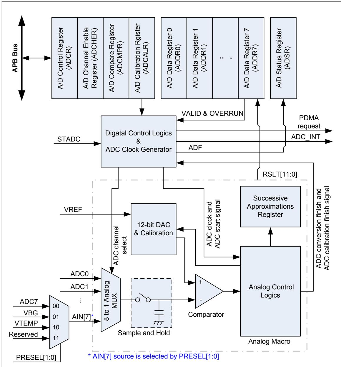
Figure 5-98 ADC Controller Block Diagram
