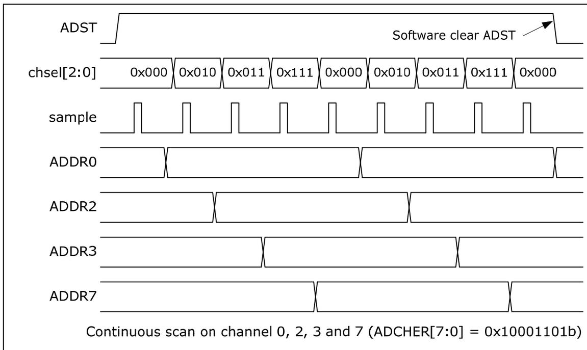
Figure 5-103 Continuous Scan on Enabled Channels Timing Diagram
