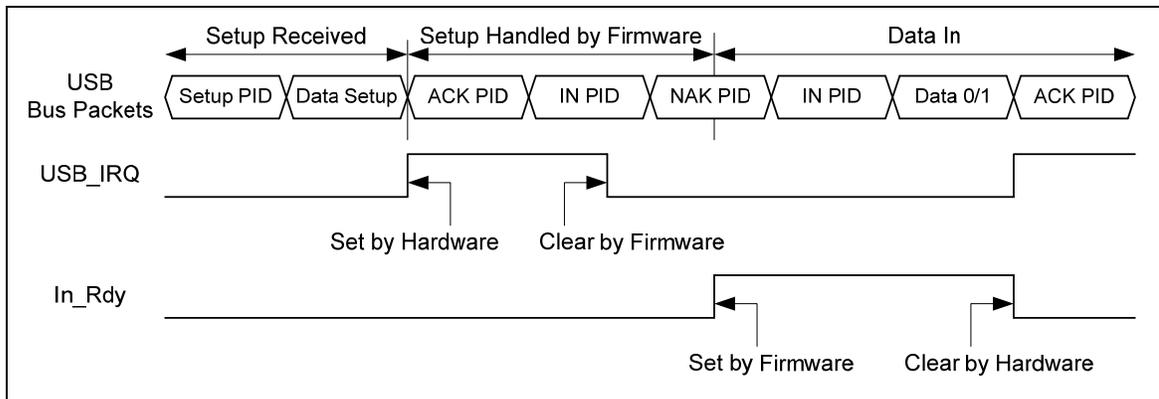
Figure 5-13 Setup Transaction followed by Data in Transaction
