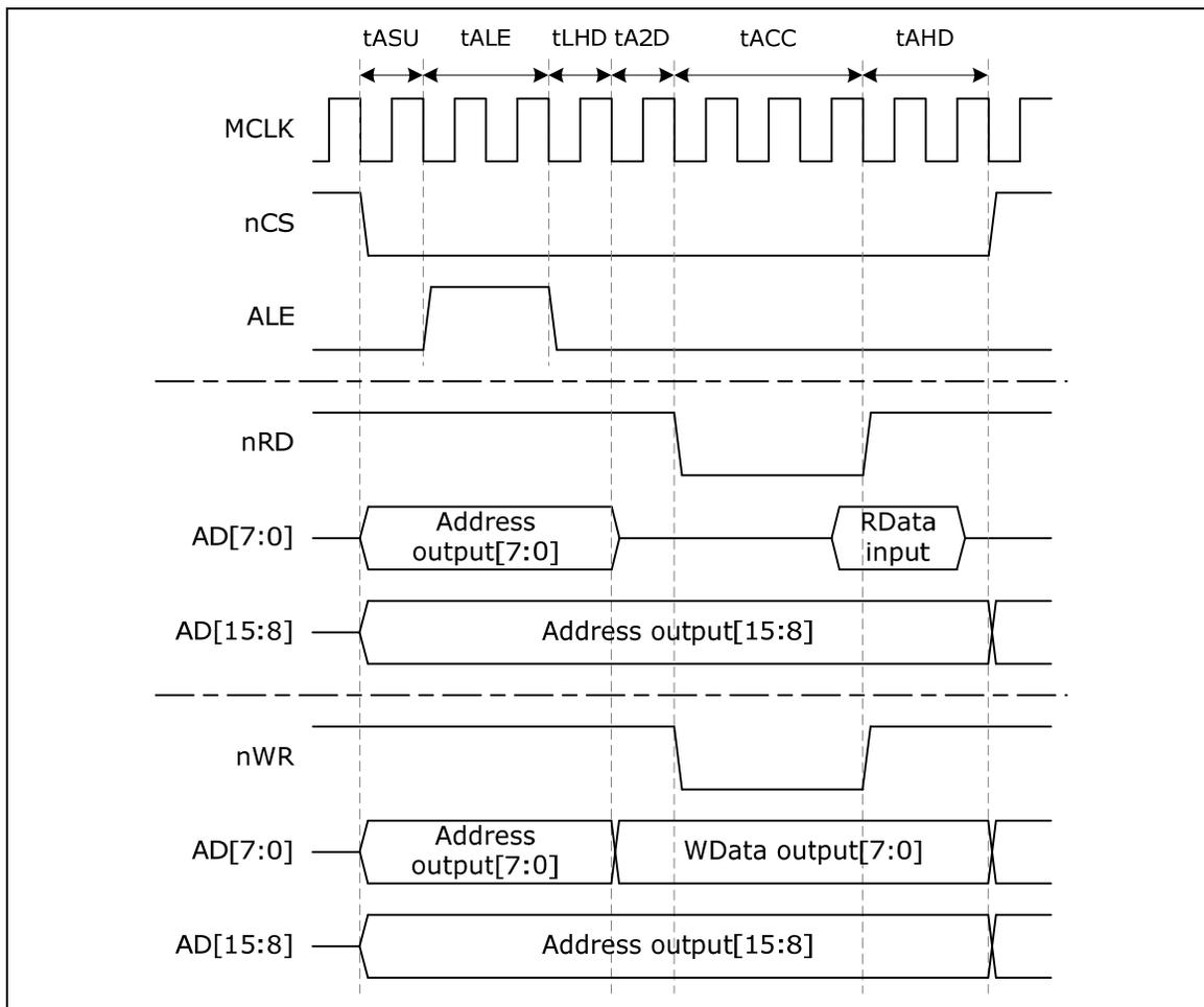
Figure 5-115 Timing Control Waveform for 8-bit Data Width
