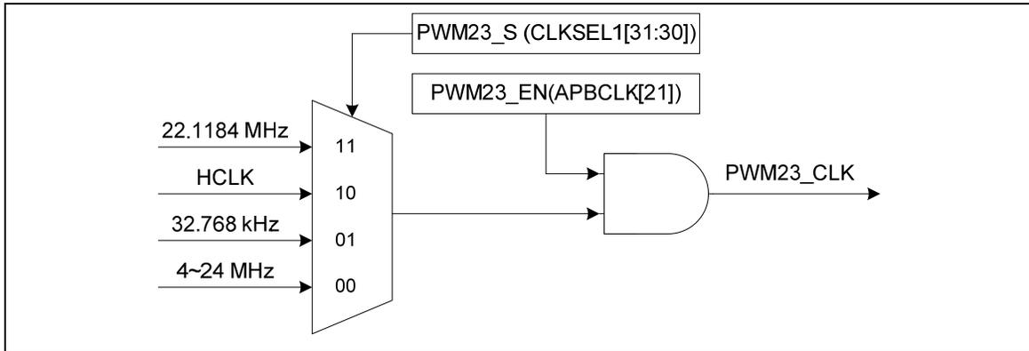
Figure 5-35 PWM Generator 2 Clock Source Control
