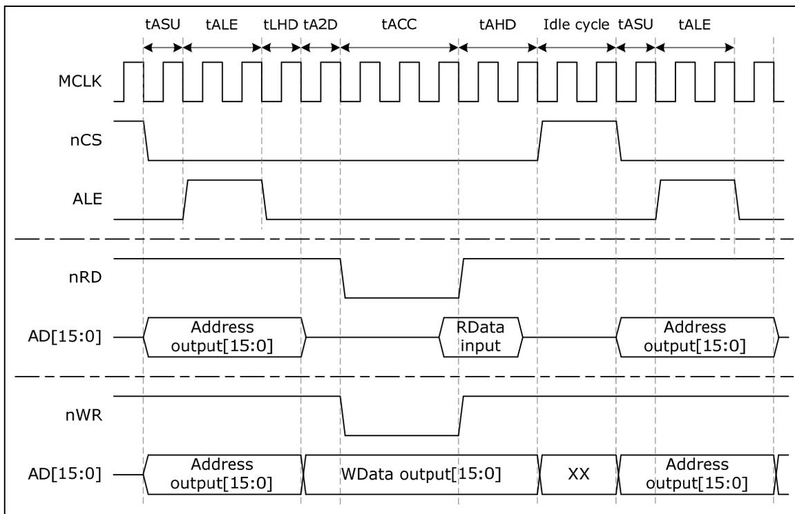
Figure 5-116 Timing Control Waveform for Insert Idle Cycle
