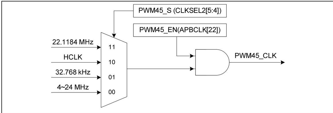
Figure 5-37 PWM Generator 4 Clock Source Control
