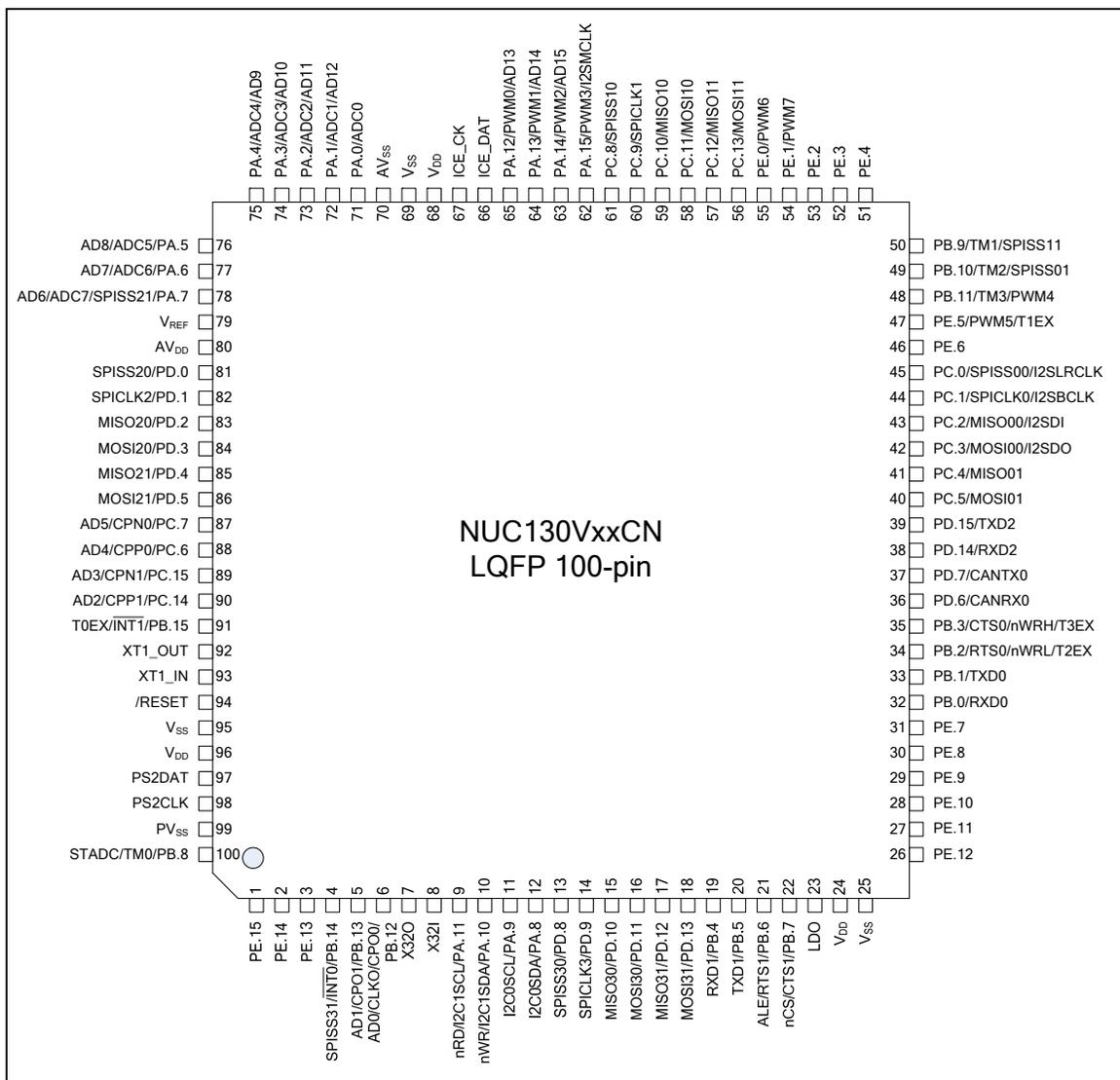
Figure 3-2 NuMicro™ NUC130 LQFP 100-pin Pin Diagram
