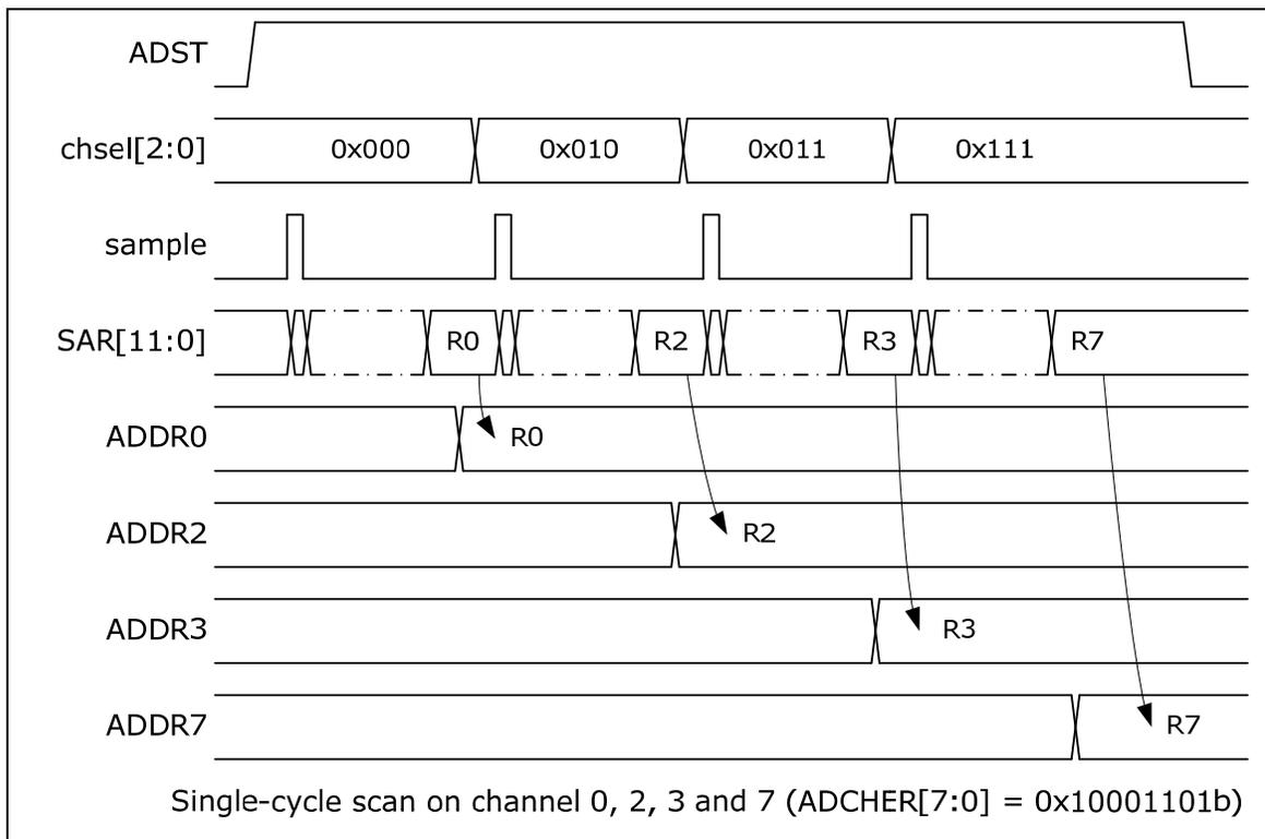
Figure 5-102 Single-Cycle Scan on Enabled Channels Timing Diagram
