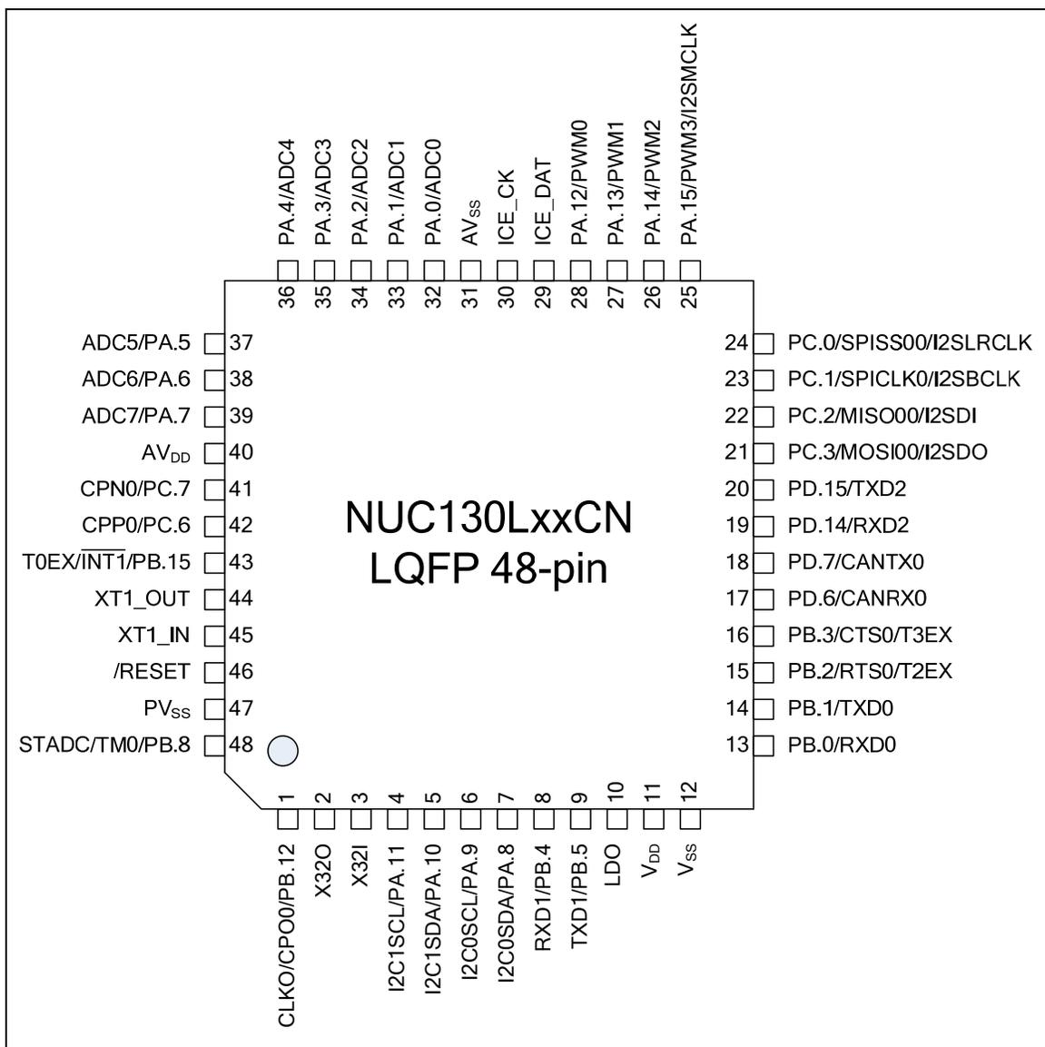
Figure 3-4 NuMicro™ NUC130 LQFP 48-pin Pin Diagram
