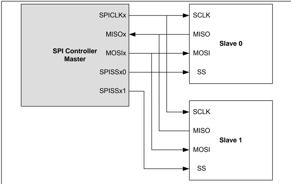
Figure 5-51 SPI Master Mode Application Block Diagram
