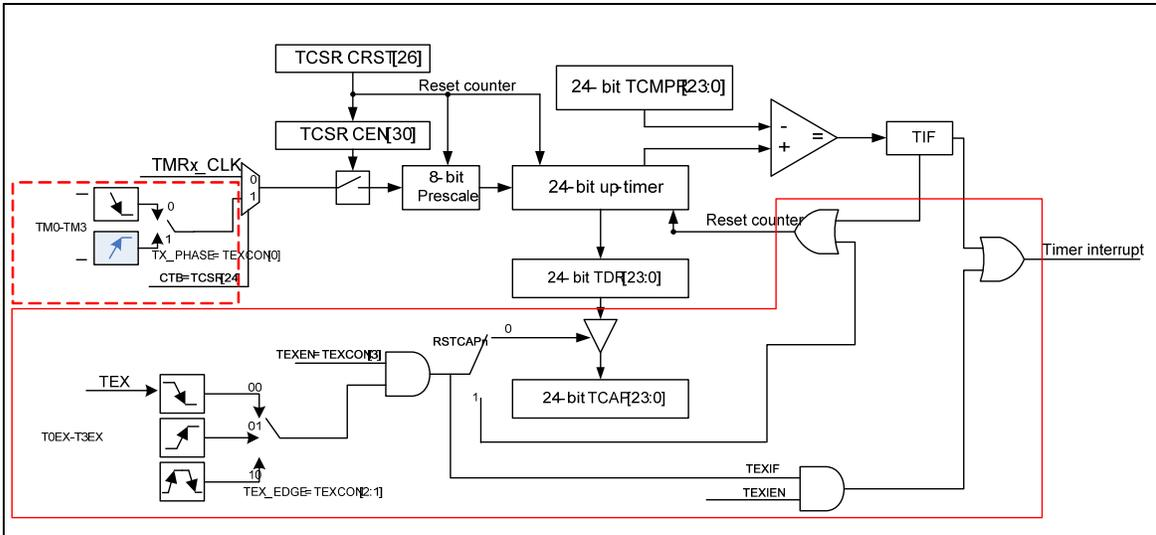
Figure 5-63 Timer Controller Block Diagram
