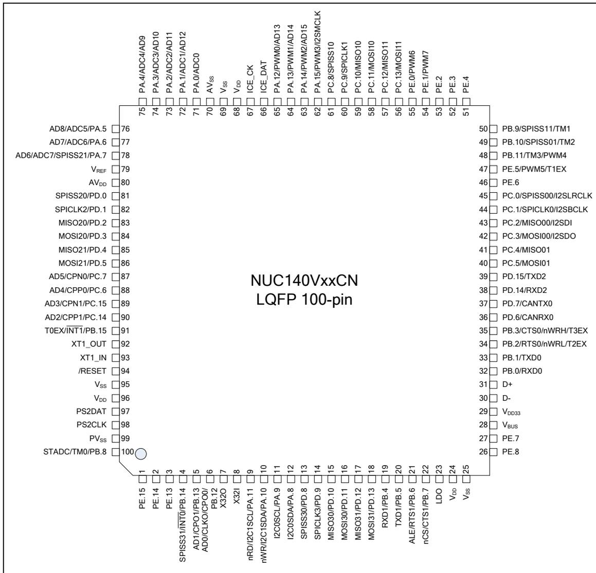
Figure 3-5 NuMicro™ NUC140 LQFP 100-pin Pin Diagram
