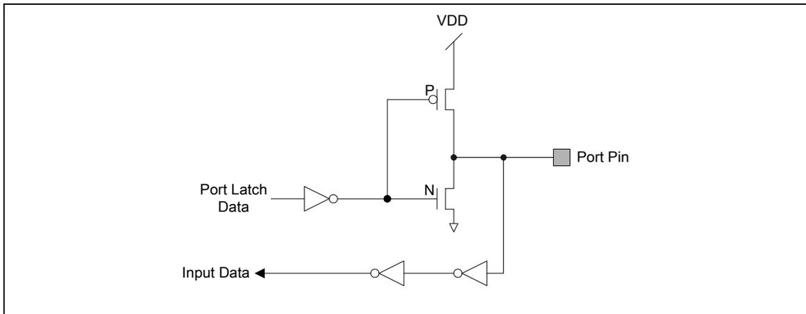
Figure 5-15 Push-Pull Output
