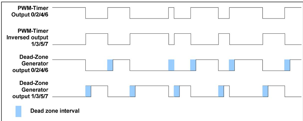
Figure 5-45 Paired-PWM Output with Dead Zone Generation Operation
