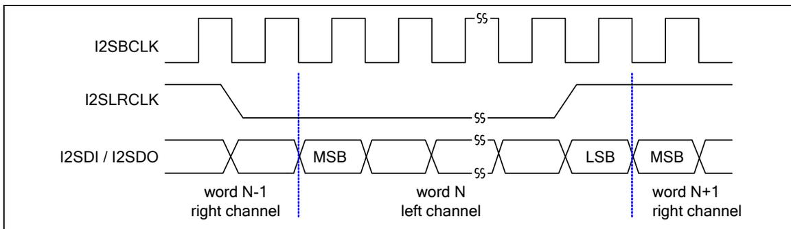
Figure 5-95 I<sup>2</sup>S Bus Timing Diagram (Format=0)
