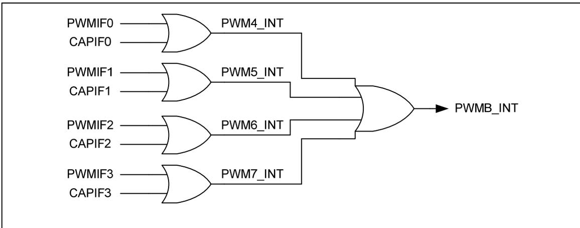
Figure 5-48 PWM Group B PWM-Timer Interrupt Architecture Diagram
