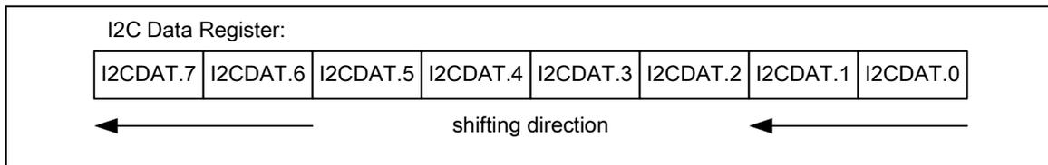
Figure 5-25 I<sup>2</sup>C Data Shifting Direction
