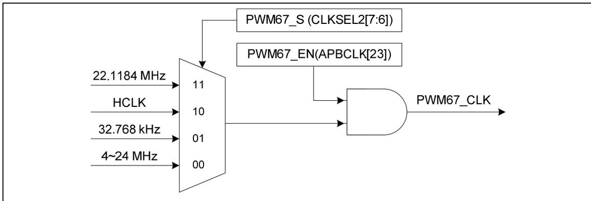
Figure 5-39 PWM Generator 6 Clock Source Control
