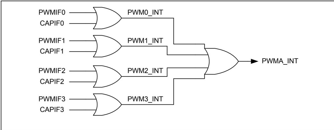
Figure 5-47 PWM Group A PWM-Timer Interrupt Architecture Diagram
