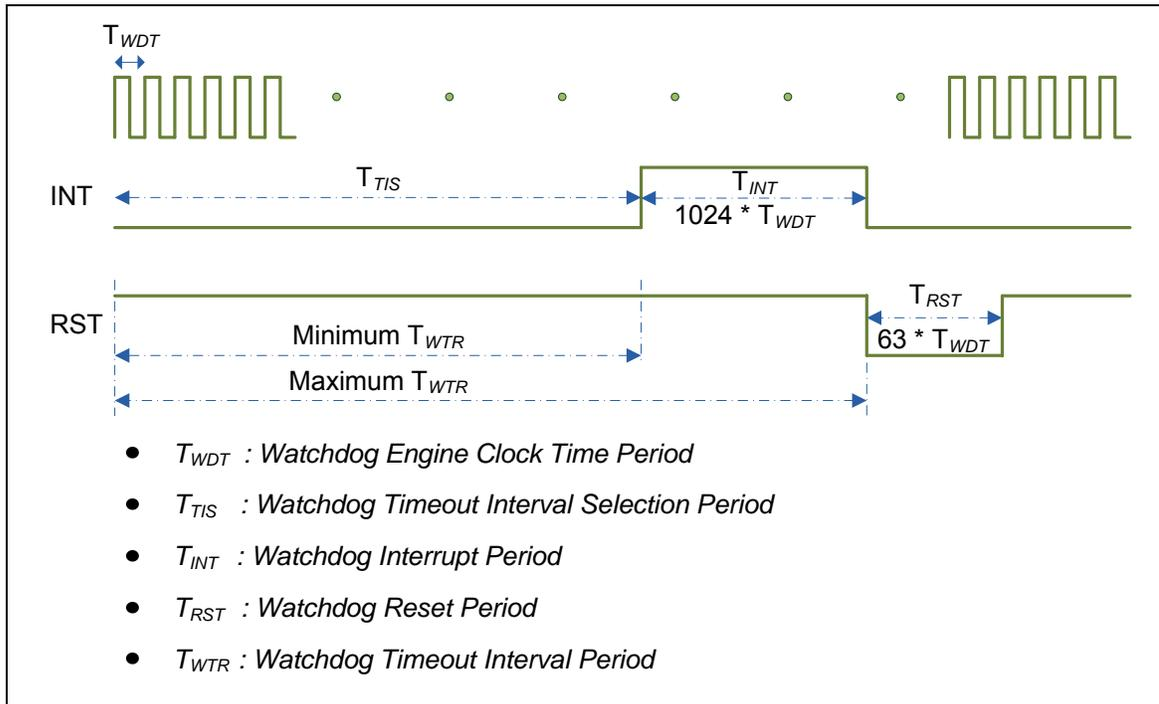
Figure 5-66 Timing of Interrupt and Reset Signal
