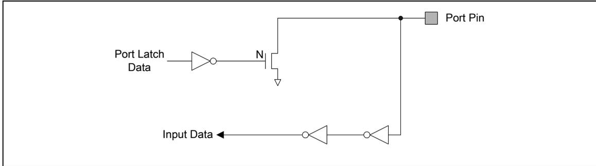
Figure 5-16 Open-Drain Output
