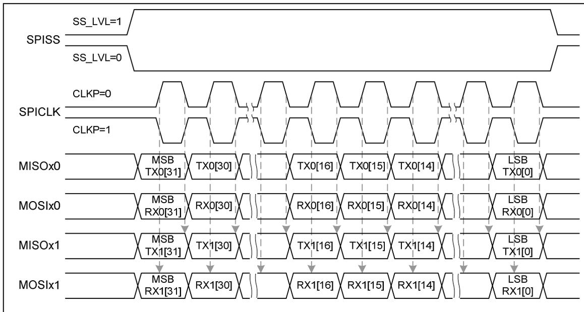
Figure 5-58 Two Bits Transfer Mode (slave mode)
