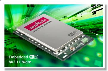
The SN8200 is a small, low power, self-contained, certified Wi-Fi® network controller module that provides simple serial-to-Wi-Fi® connectivity to the internet. It is an ideal solution for manufacturers who are looking to add wireless connectivity to home appliances or other devices for the healthcare equipment and industrial control and monitoring markets.
