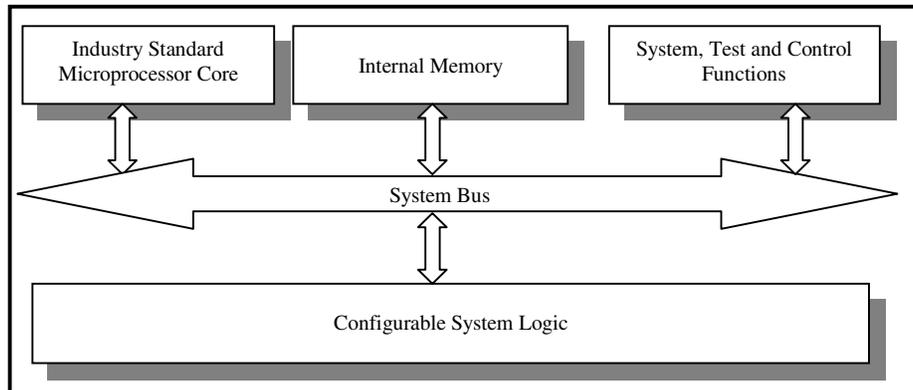
Figure 1: Basic elements and internal structure of the Triscend's CSoC.
