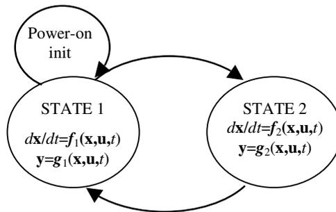
Figure 3. The state transition graph for the reconfigurable hardware.
