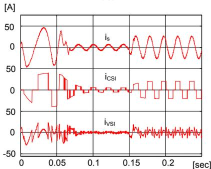
**Figure 4.** Time diagram of the tandem inverter output currents.
