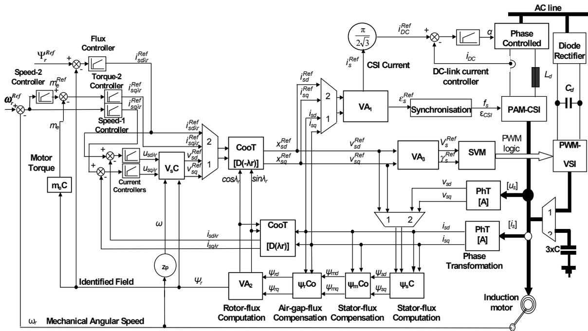
Figure 1. Rotor-field oriented vector control system for the tandem converter-fed induction motor.
