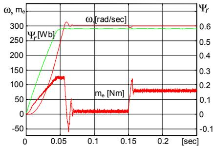
**Figure 2.** Speed and torque diagram for motor starting and load perturbations.
