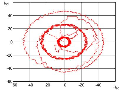
**Figure 5.** The space-phasor diagram of the stator currents.
