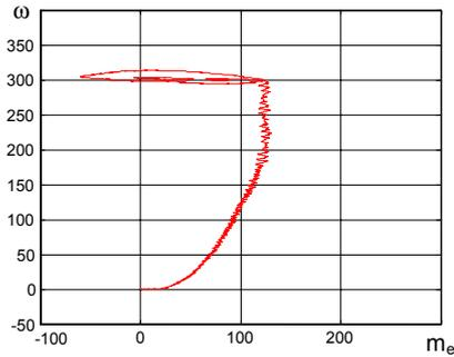
**Figure 3.** Mechanical characteristics of the induction motor.
