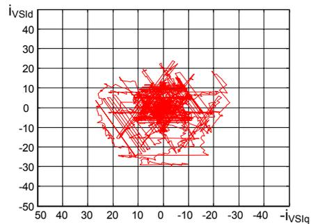
**Figure 7.** Space-phasor diagram of the PWM-VSI output current.
