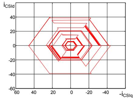
**Figure 6.** Space-phasor diagram of the PAM-CSI output current.
